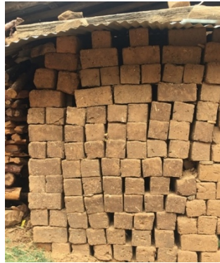
Figure 30. Dried Mudbricks stored in temporary sheds (Source: Author)
