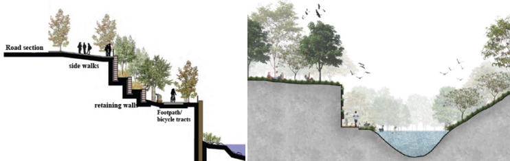
Figure 23. Retaining walls in the narrow sites (Courtesy: Hanson, 2012)
