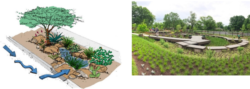
Figure 26: Green infrastructure for water infiltration (courtesy: Irienergy solution)
