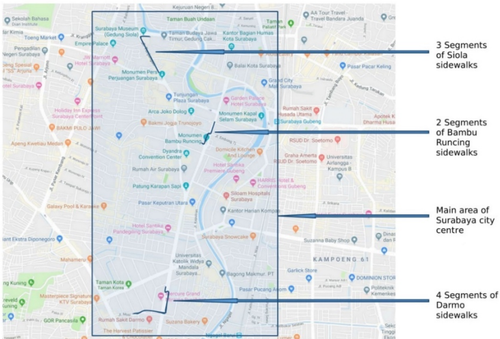
Figure 6. Map of the surveyed sidewalk segments. It consists of 9 segments, each of approximately 250 m length. Each segment represents different sidewalks condition and or different types of street-crossing methods. The area inside the box is the city center of Surabaya (after Google maps).
